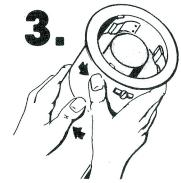
Turn collar counterclockwise until adjustment clips hold cups firmly in place. Tighten locking screw. DO NOT BEND CLIPS BY HAND!
