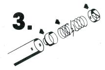
Reassemble unit by inserting cup holder, spring and bottom, making sure tabs snap into Be sure to check windows. adjustment before reinstalling.
