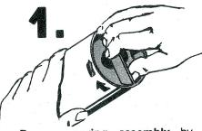
Remove spring assembly by rotating plastic base clockwise until tabs are released from Pull bottom out window. carefully.
