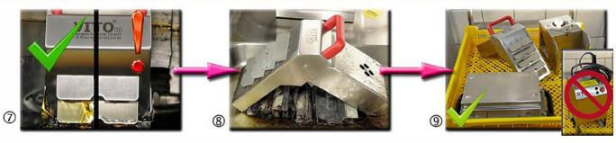
Power cord must NOT cross workspace! Tripping Hazard! Do NOT use damaged unit! Star handle screws must be tightened before every use! Do NOT touch rotating parts! Danger of injury! Do NOT move VITO during operation! Hold VITO only at the handles! After filtration Unit is hot! Danger of scalding
