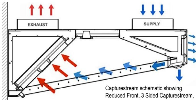
Superstream Filters - more efficient at grease capture than competitive brands and with lower air rates
