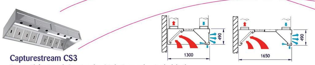
Extract with front supply & spot cooling & induction supply - standard depth
