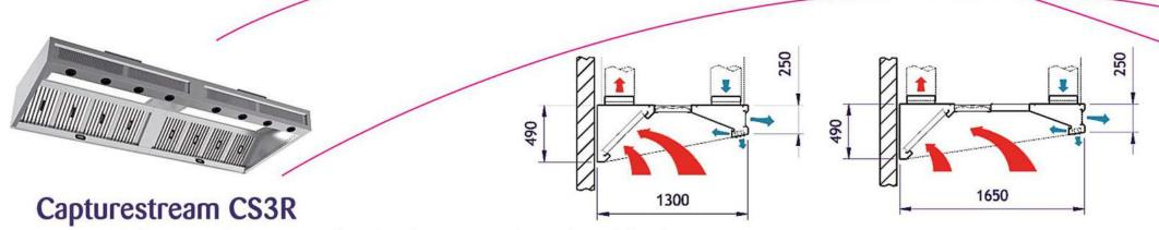
Extract with front supply & spot cooling & induction supply - reduced depth
