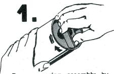
Remove spring assembly by rotating plastic base clockwise until tabs are released from window. Pull bottom out carefully.
