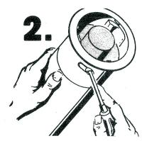
Loosen locking screw, and load cups into dispenser.
