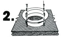
**Fasten mounting ring** securely over hole with the supplied mounting hardware.
