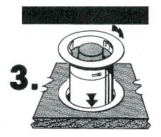
Place dispenser into hole. Align ear tabs on dispenser to openings on mounting ring. Rotate dispenser one quarter turn clockwise to secure to counter.
