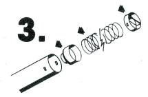
Reassemble unit by inserting cup holder, spring and bottom, making sure tabs snap into windows. Be sure to check adjustment before reinstalling.
