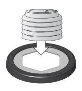
\*More delicate lids may need to be loaded into dispenser before replacing cover ring with gasket.
