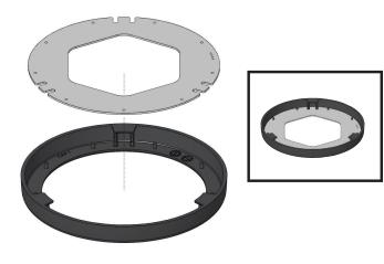
6. REPLACE COVER RINGWITH GASKET BYTURNING CLOCKWISE OVER MOUNTING RING UNTIL SECURE
