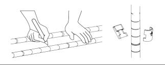
Slide the shelf with the bottom end down along 3 the post until it slides over the sleeves.
