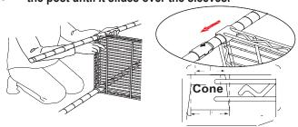
After shelf is in place, lay a piece of cloth on the 4 corner of the shelf and hit it with a rubber mallet to make it clamp tightly with sleeves.
