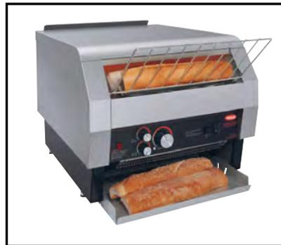
TQ Series Conveyor Toasters provide total control of the toasting of bread products. Individual controls are provided for top heat, bottom heat, conveyor speed and a stand-by switch to maximise quality and throughput. Colorgard sensing technology maintains toast quality through quiet or busy serving times. For those situations where you need to avoid patrons adjusting these controls unnecessarily, choose the TQ2 Security Cover for the TQ-805 Model.
